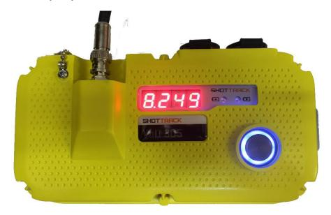
• The unit will now display 0000 which is the no cable default. If the unit is being used in a completely different location than before it might be prudent to allow an extended period to make sure a GPS fix can be acquired to set the (RTC) Real Time Clock if so then the unit can be left in this condition for 5 to 10 minutes to ensure a stable GPS fix and update the RTC. Connect the cable to the unit
